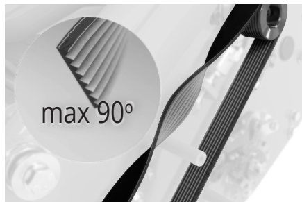
Fig.17J - Correct pressure achieved when the belt twists 90°.
