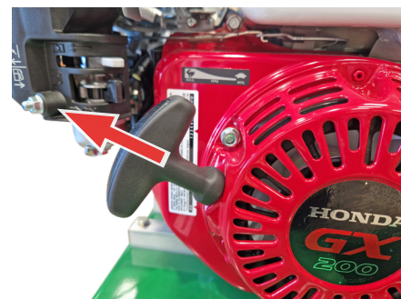
Fig.13F - Pull starter grip handle.
