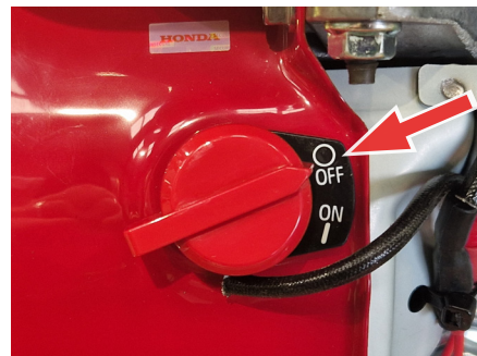
Fig.14B - Alternatively, turn the engine to off.
