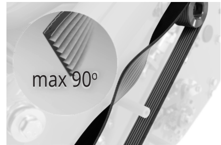
Fig.14J - Correct pressure achieved when the belt twists 90°.
