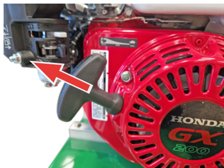
Fig.12G - Pull starter grip handle.
