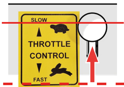
Fig.13A - Throttle set to low
