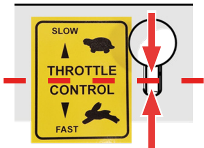
Fig.12F - Throttle set half-way
