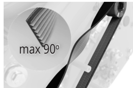
Fig. 16K - Correct pressure achieved when the belt twists 90°.
