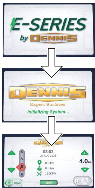
Fig. 13C - Start up sequence
