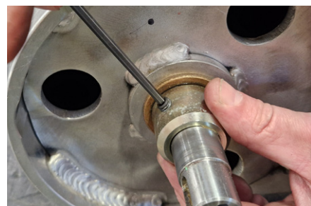
Fig. 25N - Remove grub screw
