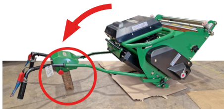
Fig. 28B - Tip the machine back. Rest on the handlebars or a block.
