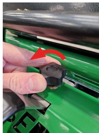
Fig. 17C - Unscrew the clamping knob.
