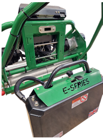
Fig. 17E - Battery removed from the machine.
