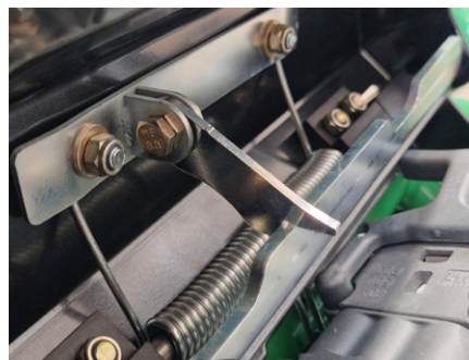
Fig. 17A - Secure the electrical box lid.
