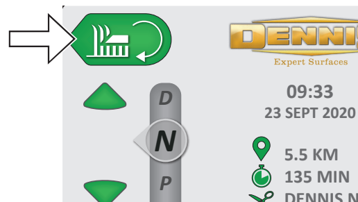
Fig. 15C - Power the cylinder unit on
