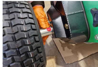
Fig. 28D - Insert the wheel axle.
