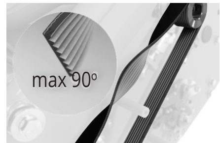
Fig. 13K - Correct pressure achieved when the belt twists 90°.
