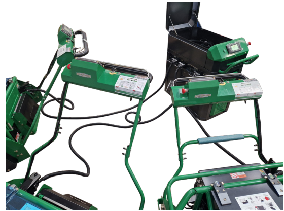
Fig.7A - Example of three machines connected to the charger.
