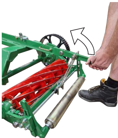
Fig.12C - Hook lift arm onto lift handle.
