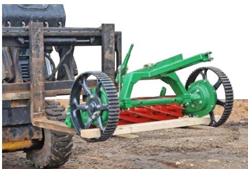
Fig.17 - Lifting method with forklift.
