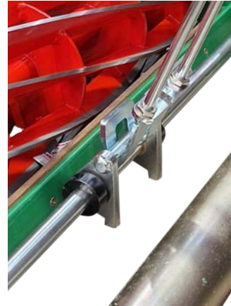
Fig.12B - Swing lift arm over handle.
