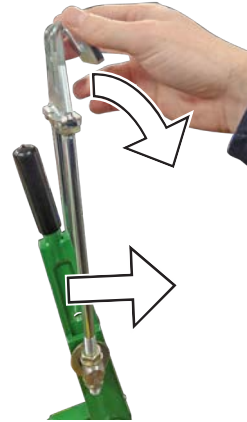
Fig.12B - Swing lift arm over handle.
