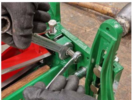
Fig.14F - Tighten lock nuts
