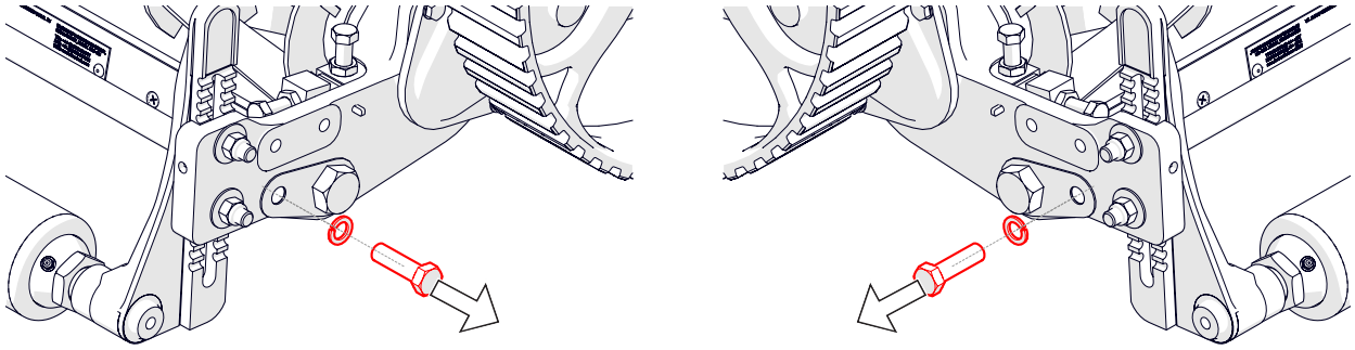
Fig.13 - Shear blade removal.
