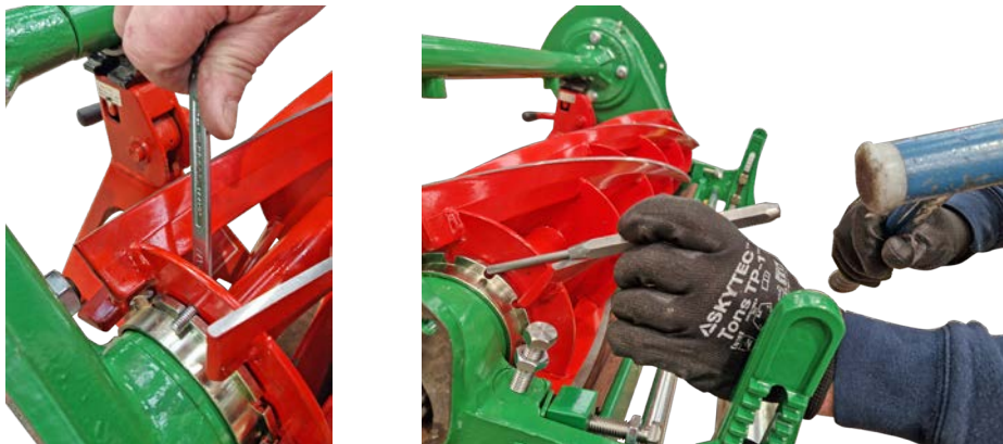
Fig.16 - Checking and tightening the cylinder bearing.
