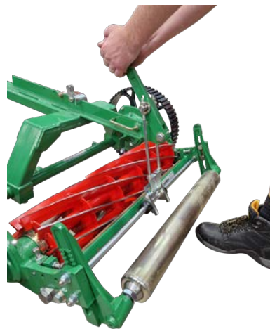
Fig.12C - Hook lift arm onto lift handle.
