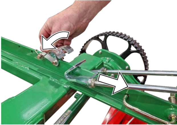
Fig.12A - Release storage catch.
