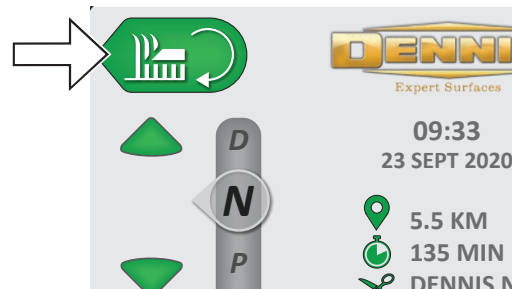
Fig. 12C - Power the cylinder unit on
