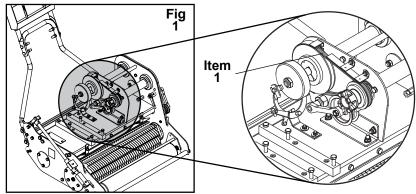
The Secondary Rear roller drive belt is shown in Fig 2 (item1). This is a hard wearing poly-V belt. Belt tension is the single most important factor necessary for long,
